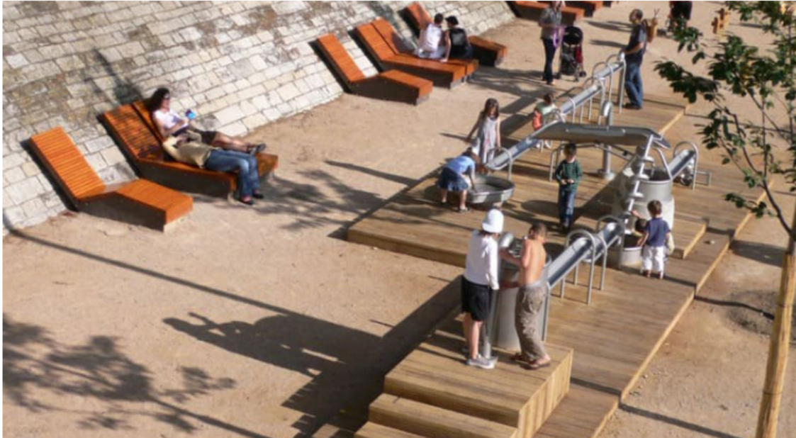
Figure 18: The playground and benches must be flood resistant with no loose fill. Water play elements need to be carefully designed as they are at high risk from flood damage.
