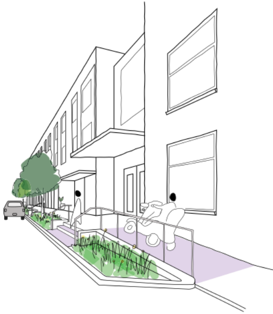
Figure 14: The raised footpath protects pedestrians from flood and enables level transitions into buildings. Steps and ramps are integrated into the streetscape with greenery. Water Sensitive Urban Design can be incorporated into the garden bed to capture and treat stormwater. Raising the footpath can encumber the flexibility of the public realm to adapt in the future and is only appropriate in certain circumstances where it has been proven to be the best solution.
