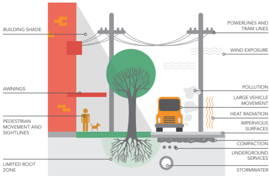
Figure 6. Illustration of common constraints for trees in urban areas. Source: Maribyrnong City Council (2018) Urban Forest Strategy.
