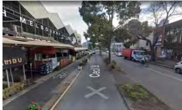
This location has low traffic speeds, median strip with pedestrian refuges, separated bike lanes, large native canopy trees, consolidated power lines, weather protection, fine grain retail mix, human scale architecture.
