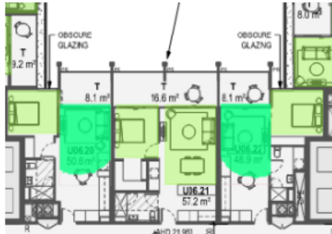
Extract from Figure 10: L06-L08 Daylight compliance area markup. This floor plan matches the advertised plans.
