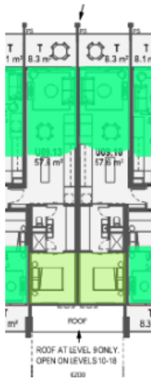
Extract from Figure 11: L09-10 Daylight compliance mark up. This matches the floor plan for levels 9 – 18 of the advertised plans.
