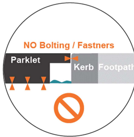
Figure 26: Structures must not be fixed to the pavement or the kerb upstands.
