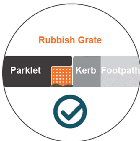
Figure 25: A rubbish grate will prevent litter from being trapped under the platform
