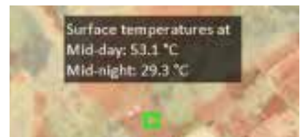
Figure 2: Aerial Thermal Images Road Surface Temperature with no shade
