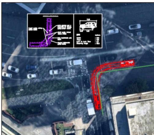
Figure 4: Swept path of a small vehicle.
