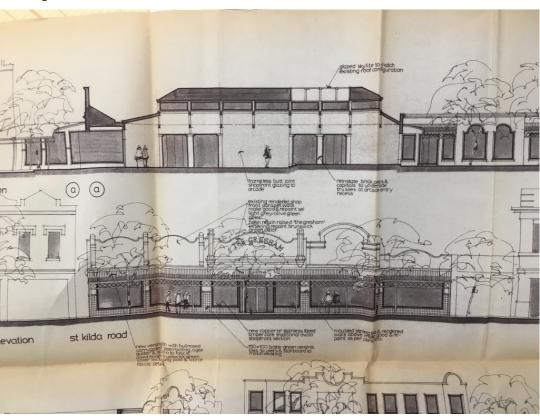
Figure 3. Plans showing retention of original parapet profiles
